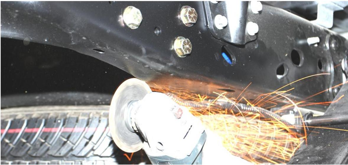
33. **NOTE:** If installing bypasses, the factory exhaust of the 2008-2016 will likely need modification shortly after the initial bend (that routes up and over the axle) to clear the bypass tubes.
